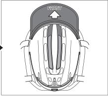
2 Attach the front visor where the front pad and top pad were attached. And press firmly hook and loop fasteners when attaching the front visor.
