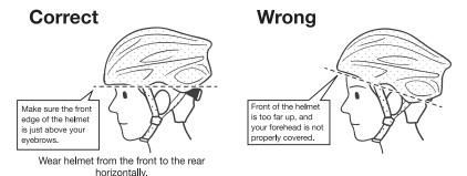
By wearing the helmet properly and fastening chin strap securely, it is possible to maximize the protecting functions of your helmet in the event of an accident. Therefore, wear your helmet properly before riding.
