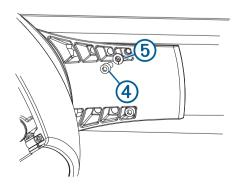
**4** Torque the hex bolts to 0.81 kgf-m (70 lfb-in. [6 lbf-ft.]) to fasten the antenna to the pedestal without damaging the antenna or the mounting hardware.
