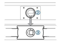
**3** Secure the antenna to the pedestal using the included hex bolts ④ and spring washers ⑤.
